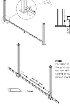
For shorter sections, cut the top rail to fit between the posts minus 5/8" for the bracket depth. For the bottom rail, subtract 5/16" from each end after taking an overall measurement to ensure equal picket spacing.
