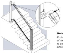
Push the top rail into the bottom of top stair bracket, screw top rackets to rail using 2 #8-3/4" pan head self-drilling screws.
