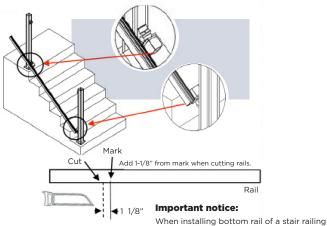
section, remove the vinvl insert, and install in opposite direction as shown:
